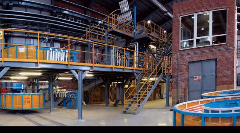
phosphorous bronze and after obtaining the desired alloy, the melt is transferred to a 7 ton holding furnace. Then, through UPCAST, primary mother tubes with 38/33 and 52/47 (OD/ID) dimensions are drawn directly and transferred to the special baskets.
