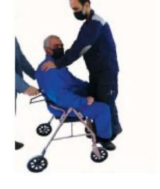
Maximum load test with 150 kg while working mode wheelchair
